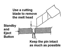
1. Remove the original button assembly by cutting the melt point as shown
